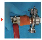
Wrap firmly at least one time plus two to three centimeters around pipes, flanges, valves, etc. and tear it with your fingers. Press firmly to secure the edges. There is no need for scissors or any adhesives. The band can be removed and reapplied several times if necessary. Replaced the band when the color has faded.
